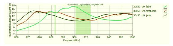
Sensitivity&Read Range Test power: 4W EIRP
